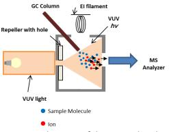
Figure 2. Schematic of the PI ion chamber.
