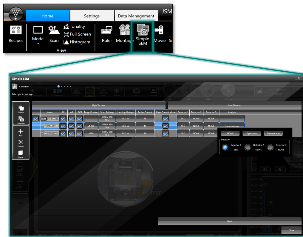
Figure 1. Simple SEM is fully integrated within JEOL's SEM control software, creating an intuitive environment for users to develop automation workflows without any need for programming experience.
