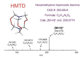
Figure 2. AccuTOF-DART mass spectrum of HMTD
