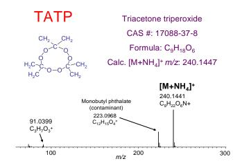
Figure 1. AccuTOF-DART mass spectrum of TATP
