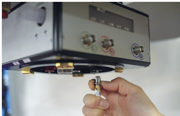
Adoption of a single-touch quick coupler made coupling and decoupling the probe from the Auto Tune Unit easy.
