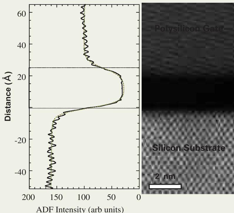
Fig.6. Quantitatively measuring the thickness of a 2.5 nm gate oxide from an ADF image. The gaussian interface roughness model fit is shown as a dotted line. The lower and upper interface roughnesses were 1.75 Å and 3 Å rms respectively. The inner semi-angle on the ADF detector is 40 mrad and the probe forming aperture was 10 mrad semi-angle. (Digiscan and JEOL 2010F-ARP)
