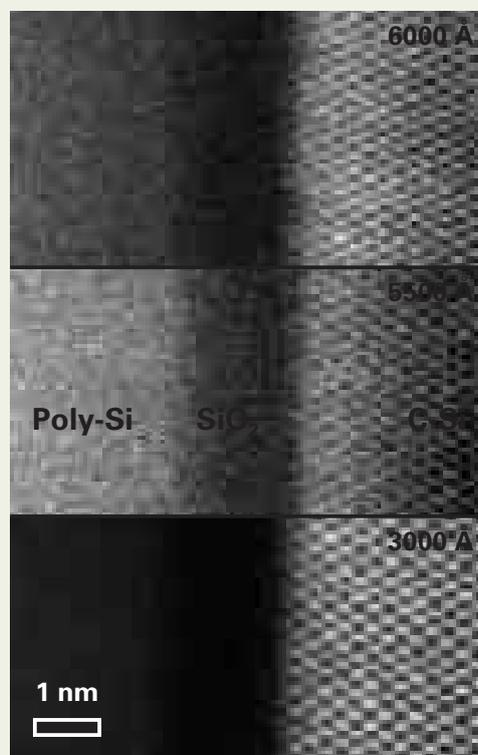
Fig.5. ADF images of a 2 nm gate oxide recorded at different sample thicknesses. The inner semi-angle on the ADF detector is 40 mrad and the probe forming aperture was 10 mrad semi-angle. The main effect of sample thickness is a reduction in signal/noise. The sample thickness was determined by EELS. (Digiscan and JEOL 2010F-ARP)
