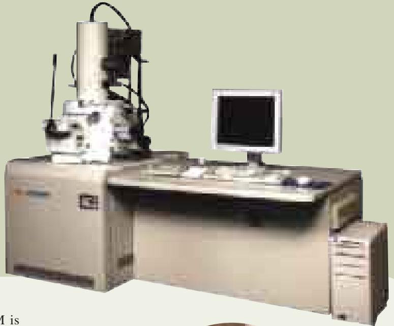
JSM-6500F multi purpose high performance FE SEM is equipped with the newly developed In-Lens Thermal FEG, unique combination of the thermal FEG (Field Emission Electron Gun) and the condenser lens produces high probe current sufficient for EBSP, WDS and CL analysis as well as high magnification image observation and EDS. A high probe current in a very small electron probe size enables one to analyze smaller area.
