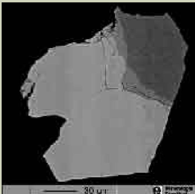
Fig.4. Backscattered electron image of the polished surface of the Ca-silicates in diamond KK-44. Two crystals of larnite ( $\text{Ca}_2\text{SiO}_4$ ) form the bright coloured left part of the inclusion. The darker coloured upper right consists of  $\text{CaSi}_2\text{O}_5$ -titanite. The darker veins within the brecciation are chemically not distinct from the host. The thin grey band separating larnite and  $\text{CaSi}_2\text{O}_5$  consists of  $\text{CaSiO}_3$ .
