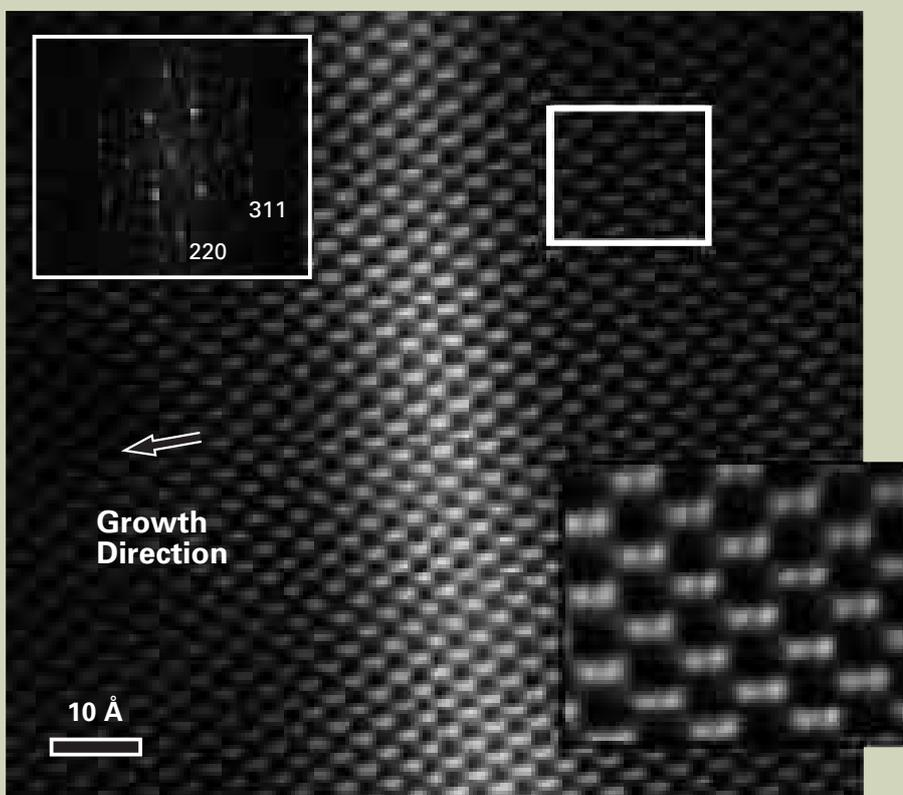
Fig.3. Bright Field STEM image of a gate oxide recorded with the Emispec system. The interface roughness was roughly 8 Å peak-peak (or 1.7 Å rms). The collection semi-angle was 1 mrad, and the probe forming aperture was 10 mrad semi-angle. (Emispec and JEOL 2010F-ARP)
