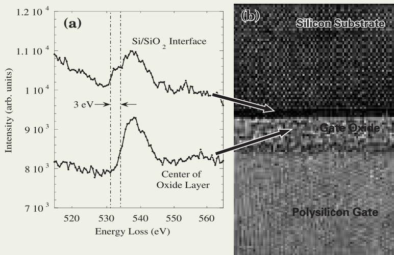
Fig.4. The HRTEM image recorded in the JEOL 2010F showing the 2 nm thick gate oxide and used to position the probe for spectroscopy. A Gatan imaging filter was used as the spectrometer, as the photodiode array of a conventional PEELS is not sensitive enough to detect the energy losses from a 20 pA, 0.2 nm sized probe. The interface states are visible as a pre-peak 3 eV below the O-K edge. This implies a reduced energy gap at the Si/SiO<sub>2</sub> interface [4].
