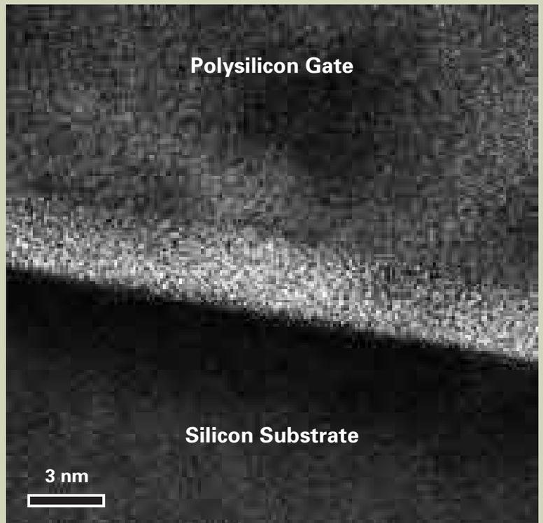
Fig.2. Annular dark field STEM image of an antimony delta-layer in [110] oriented Si, showing an information limit better than 0.163 nm, and minimal drift during the 40 second acquisition. The peak antimony concentration is 20 atoms or about 0.2 monolayers. (Digiscan and JEOL 2010F-ARP)
