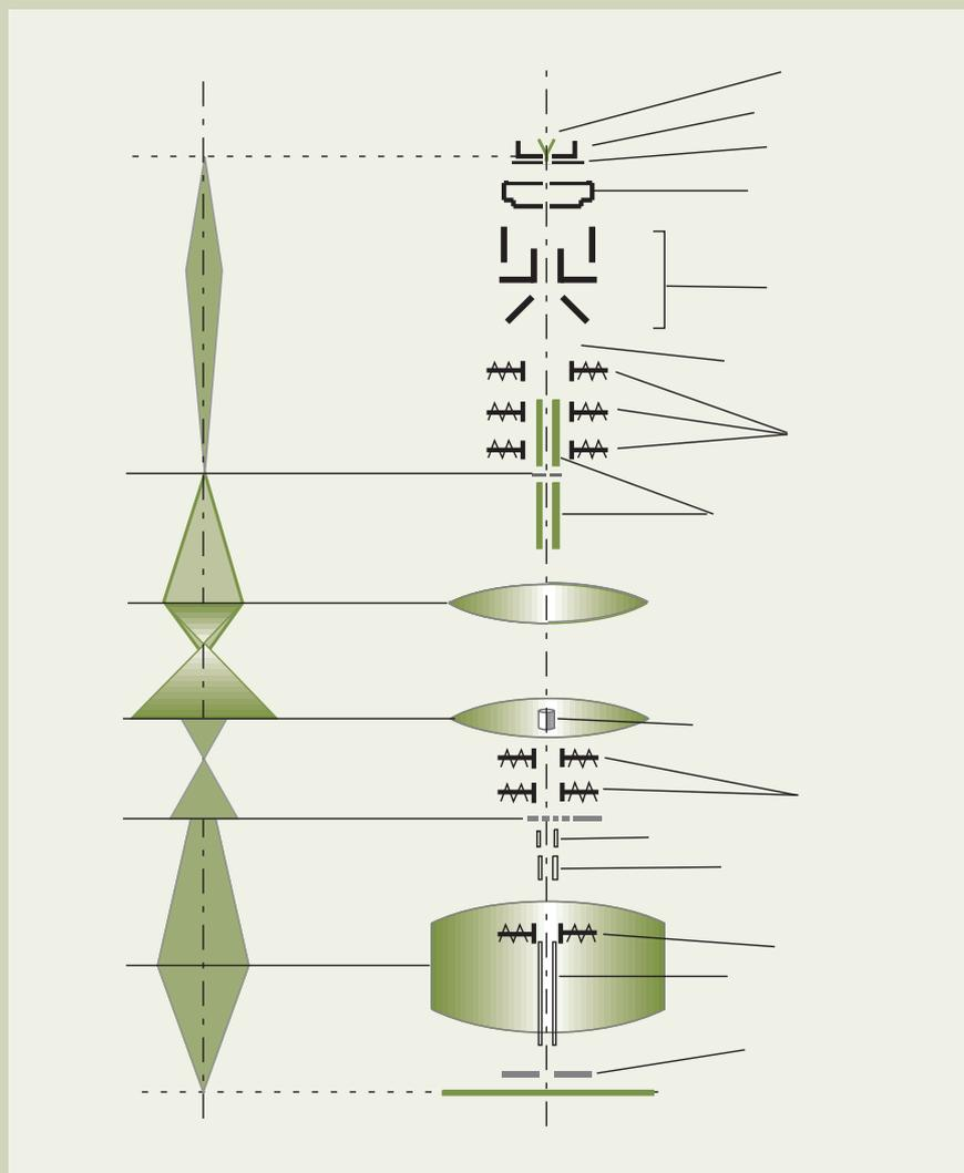
Fig.2. Electron optics system of JBX-9300FS.
