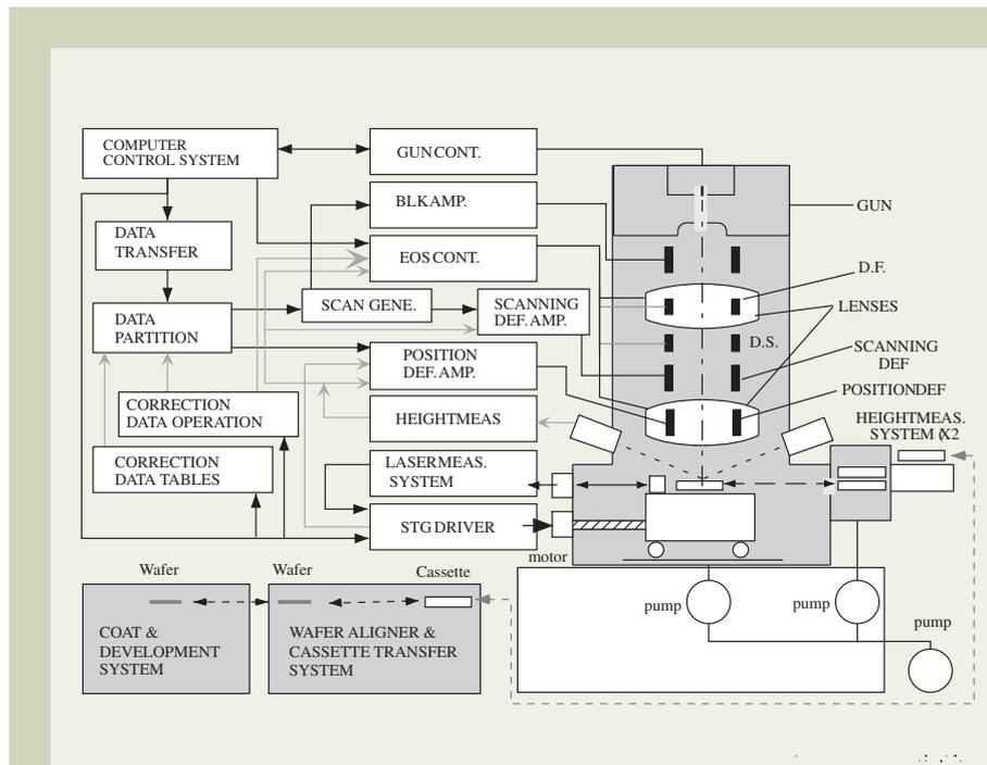
Fig.3. Block diagram of the JBX-9300FS's control system.
