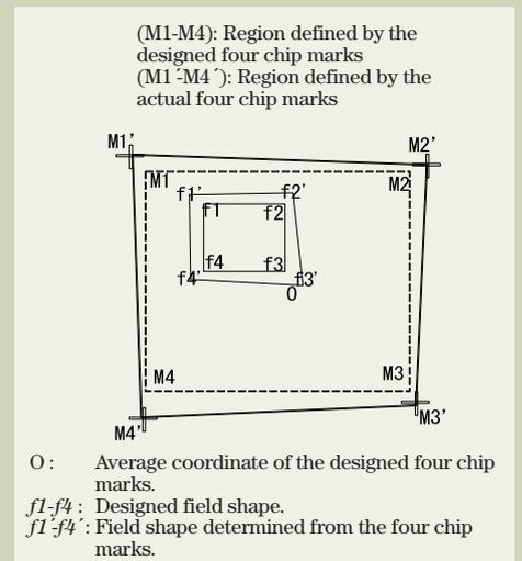
Fig.5. 4-chip marks alignment.
