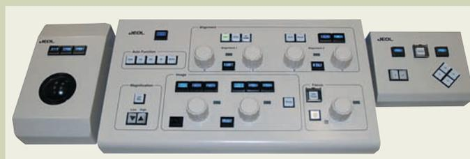
Fig. 2 Operation panels of JEM-2800. Trackball panel, main operation panel and specimen height and tilt control panel are shown from the left-hand side. Main operation panel upper-side is used for alignment, and bottom-side is used for acquisition setting of images.
