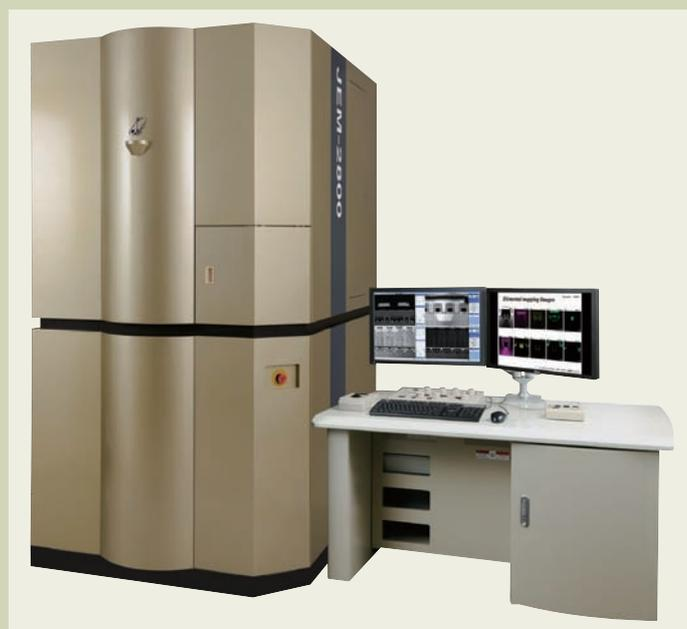
Fig. 1 External view of JEM-2800. Left-hand side of the figure is the microscope column in enclosure. Enclosure height is about 2.6 m. Right-hand side of the figure is an operation console. All operations are performed from the operation console.
