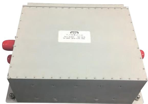
Diplexer combiner with 90dB of isolation between the  $^{19}\text{F}$  and  $^1\text{H}$  channels.
