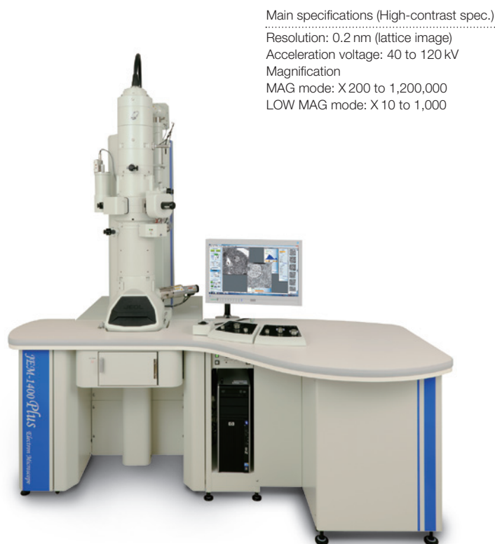
Fig. 1 JEM-1400Plus appearance and specifications
