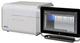
A brass pipe used for water-cooling showed cracks which resulted in water leaking. Using **ED-XRF**, we conducted elemental analysis at the crack defect and also away from the defect area. The elemental analysis results reveal that there is a difference in the content of Sn and Pb. Since the element distribution in the cracked part differs from the normal area, we conducted additional tests using EPMA.
