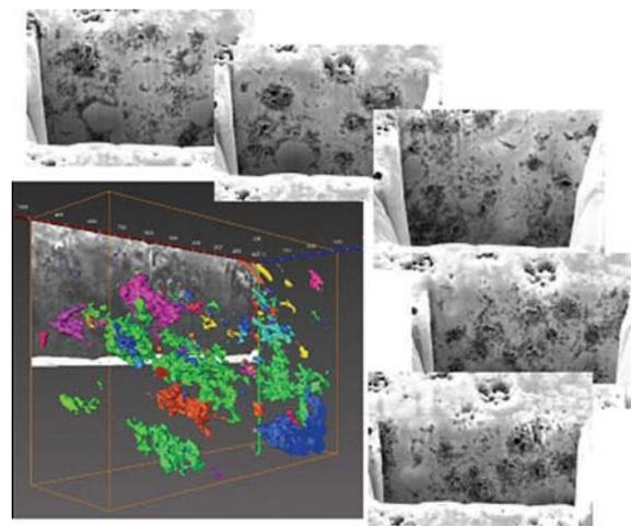
**Fig. 4** — Five out of 40 slices used to reconstruct a 3D volume of shale with the JIB-4600F FIB-SEM. A 3D rendition of the pore structure was done with Avizo software (from VSG).
