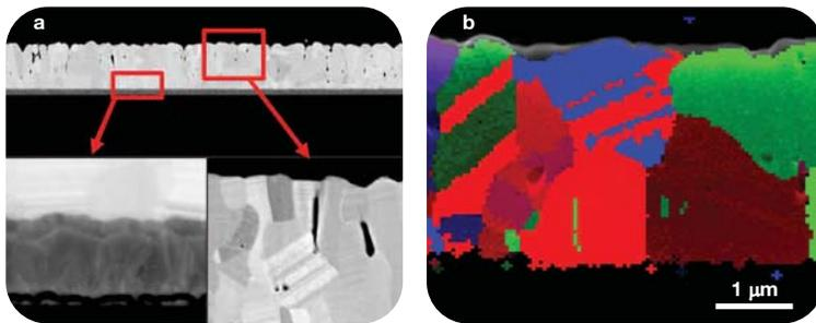
**Fig. 1** — (a) Solar panel thin film cross-section prepared with the CP. Insets show higher magnification images of the different layers of the film, with a clear view of the layer thickness and grain structure. (b) EBSD grain orientation map of the film structure.
