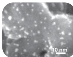
**Fig. 5** — Energy filtered image of a catalyst with sub 5 nm Pt/Pd metal particles imaged at 1,000,000X magnification.
