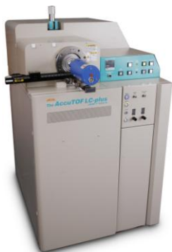
LC and Ambient Ionization HRTOF Mass Spectrometer JMS T100LP AccuTOF-DART™
