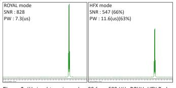
**Figure 2.** <sup>1</sup>H signal to noise and pw90 for a 500 MHz ROYAL-HFX Probe in single and dual-tune illustrating the expected changes in performance when switching modes.
