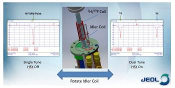
**Figure 1.** Illustration of magnetic coupling technology as a perfect switch between single tune and dual tune modes in the ROYAL-HFX Probe.
