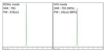
Figure 3. <sup>19</sup>F signal to noise and pw90 for a 500 MHz ROYAL-HFX Probe in single and dual-tune modes.
